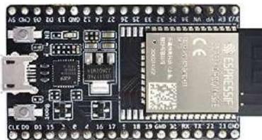
Figure 2.5: ESP32 Development Board.
