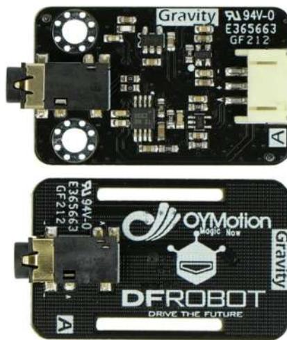
Figure 2.1: OyMotion Gravity Dry EMG Sensor.
