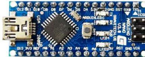
Figure 2.4: Arduino Nano Board.
