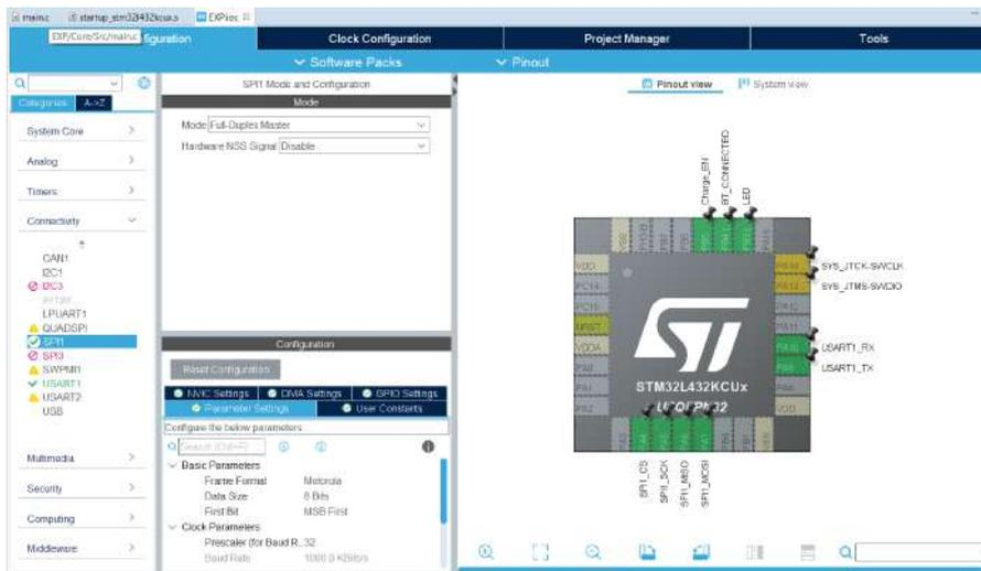
Figure 3.1: CubeMX code configuration tool.
