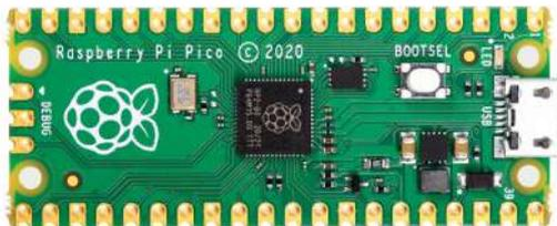
Figure 2.7: RP2040 on Raspberry Pi Pico Board.
