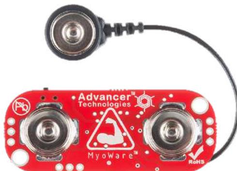
Figure 2.2: Advancer MyoWare EMG Sensor (without gel pads).
